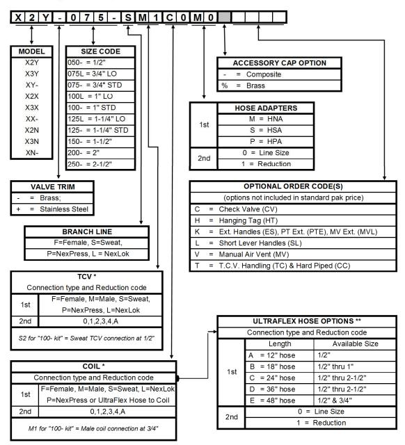
\* Please consult individual component spec sheets and/or the Union End Connection Size Guide to determine exactly if desired reduction size and connection type is available.
